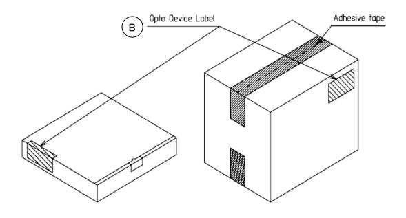
Type A Material / box : Cardoard C5BF Type B,C Material / box : Cardoard K5AF Partition : Cardoard K5BF
