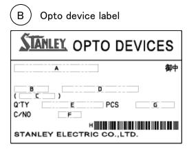
A. Custmer Name B. Parts Type C. Parts Code D. Parts Number E. Packed Parts Quantity F. Carton Number G. Shipping Date H. Bar-Code for In-house identification Number
